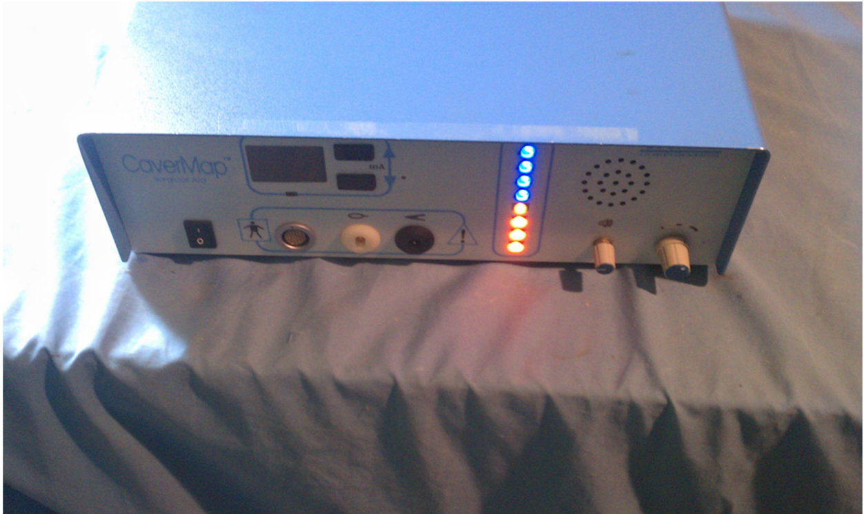
Figure 5 The CaverMap Surgical Aid nerve stimulator control unit. Device control unit with connectors for the stimulation needle, display of the applied current in mA, and LED display (blue and red) to visualize tumescence response on an ordinal scale.
