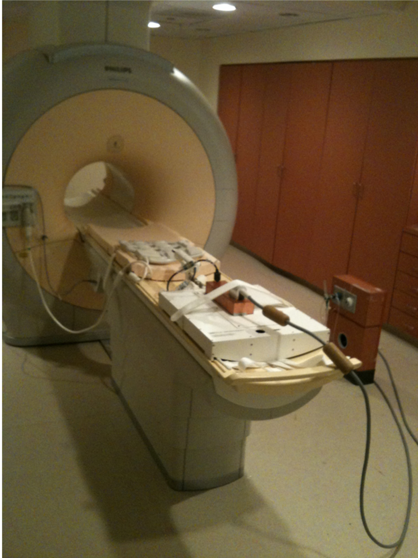
Figure 3 Equipment integration for MRI-guided ultrasound therapy. Frontal oblique view of the 3T Philips MRI scanner with an 8-channel cardiac MR coil on the anterior part of the scanner table and ultrasound transducer on the posterior part of scanner table.
